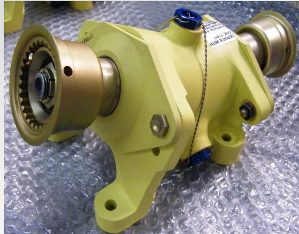
*Torque Converter Assembly*
