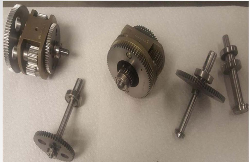
***PN 65661-11250-045 Positioner Gear Assembly for the Main Blade Gearbox CH-53***
