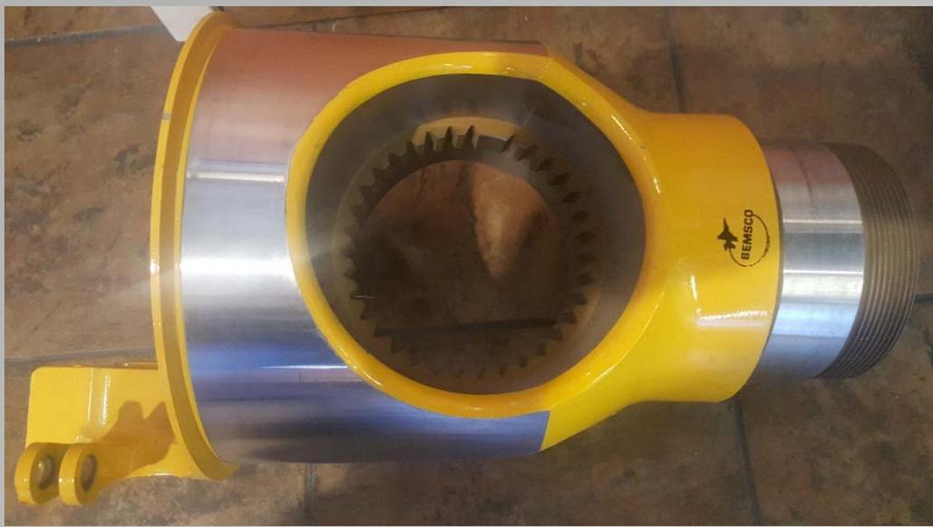
*Trunnion Assembly for KC-135 Landing Gear*
