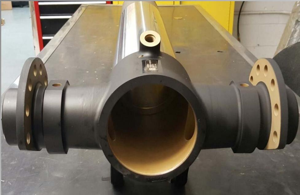
***Piston Housing for the CH-53 Nose Landing Gear***
