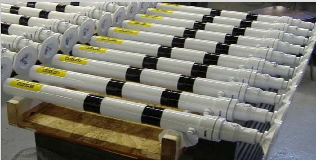
*Rammer Cylinder Assembly for M-901 Tank*
