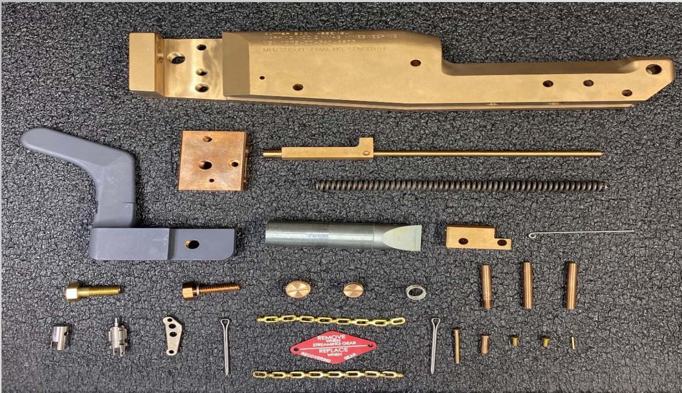
***PN 201309302 -101 DOWN LOCK ACTUATOR FOR THE F-16 NOSE LANDING GEAR***
