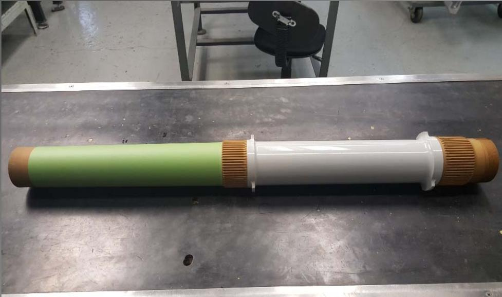
***Torque Tube Assembly for the 767***
